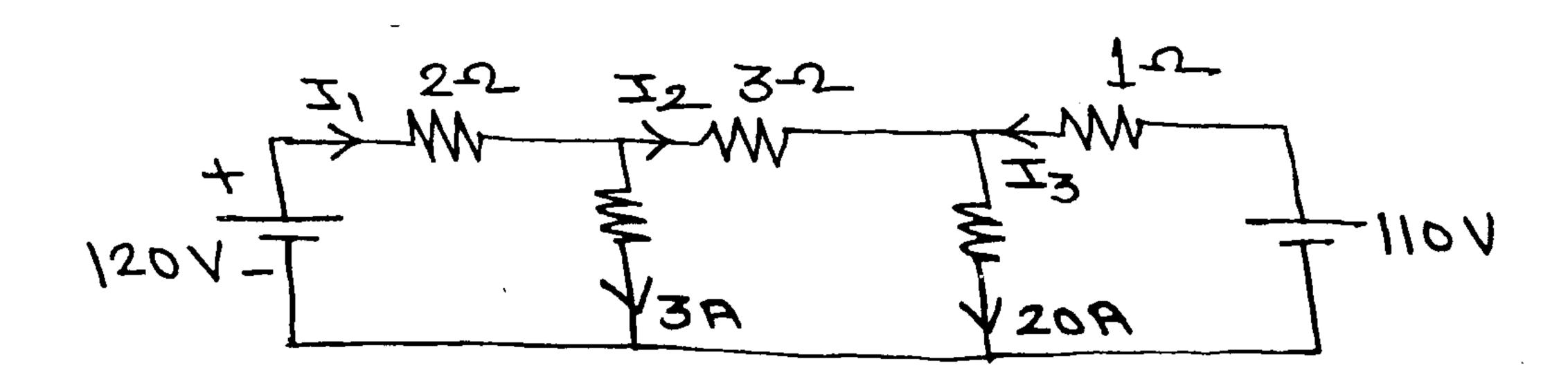
Find the currents  $I_1$ ,  $I_2$ ,  $I_3$  in the given circuit by node yoltage method.
